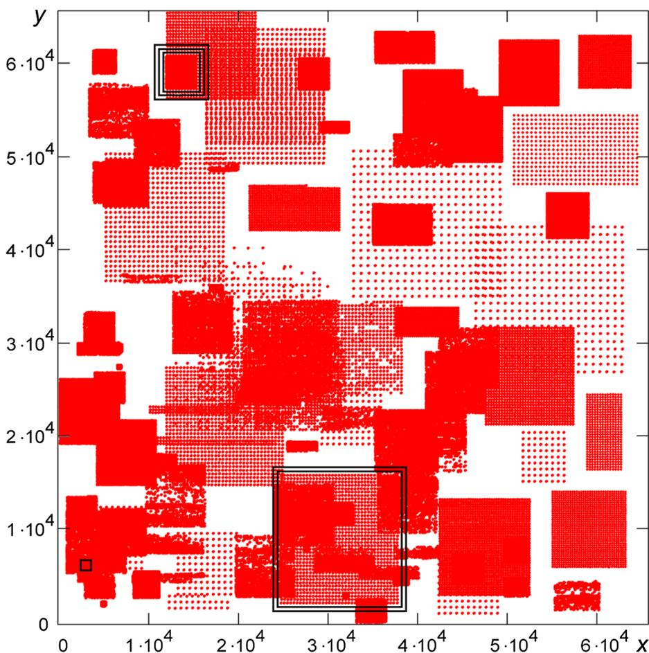
**Fig. 1.** Areas covered by distributed calibrations. The red points “•” designate the LCS positions for which LCCs were found. The x and y axes are graduated in lateral positions of the scanner. The whole scanner field is approximately equal to  $2 \times 2 \mu\text{m}$ . The calibrations have been conducted at the position of the scanner Z manipulator extended to the middle of its range.
